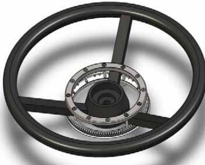
4. Tighten screws with a hex key until the main gear and ring fit snugly to the steering wheel. Tighten the screws in a cross-pattern (as opposed to tightening each screw in a clockwise or counter-clockwise order).
