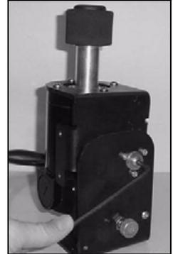
6. Apply some molybdenum sulphide grease or black grease to the exposed shaft and bearing face.
