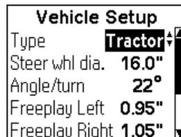
**Note** – If the **steering wheel diameter** value listed for your vehicle model is incorrect, measure and enter the correct diameter. See Appendix B: Measuring Vehicle Parameters.
