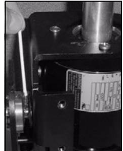
10. Ensure that the two grub screws on the steering motor output shaft are tightened to 2.8 Nm-3.4 Nm (25 in/lb-30 in/lb).
