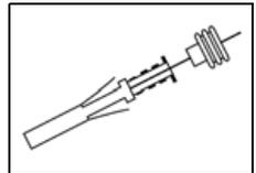
5. Insert the two female terminal connectors and the rubber seal into the two holes of the 2-way female connector as follows:
