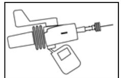
6. Plug the 2-way female connector into the 2-way male connector on the accessory cable.
