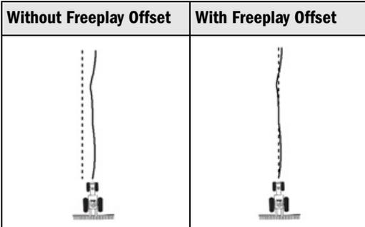
Adjust the *Freeplay Offset* value to remove steering bias.
